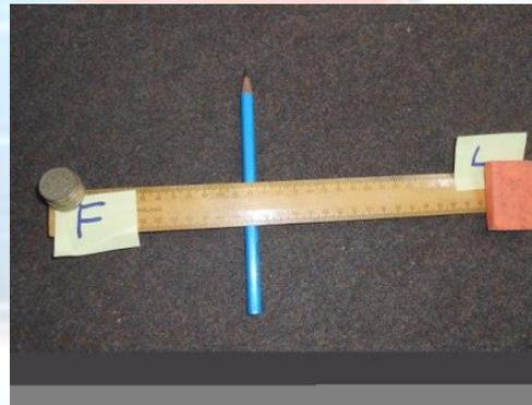
**Pattern-seeking – How much force is required when the fulcrum is in different place to lift a mass at the other end?**
