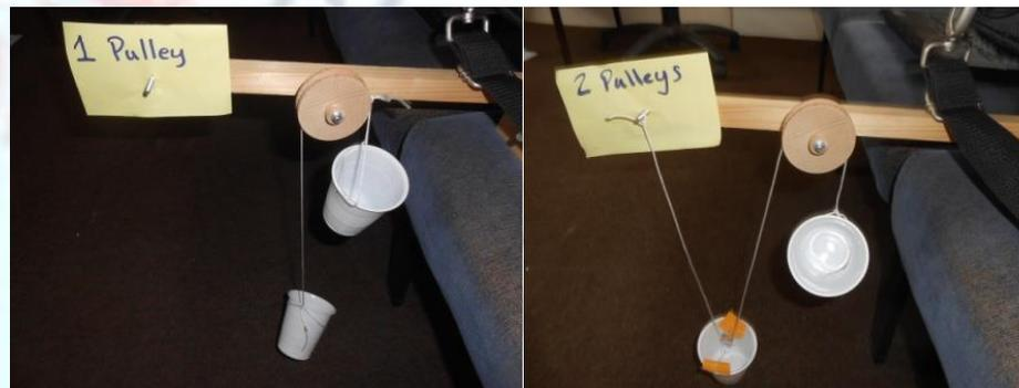
Challenge the children to find out how much mass must be placed in the top cup to make the one at the bottom lift off the ground. They can begin with no pulley by simply placing the string over the wooden pole. They can then try one and then two pulleys.
